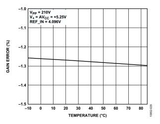
Figure 12. Gain Error vs. Temperature
