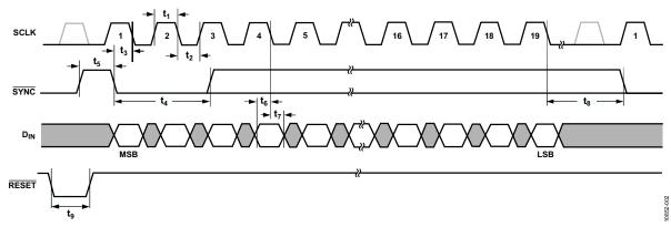
Figure 2. Serial Interface Timing Diagram
