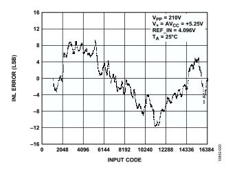
Figure 6. INL with Full-Scale Range = 200 V
