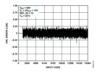
Figure 5. Differential Nonlinearity (DNL) with Full-Scale Range = 50 V
