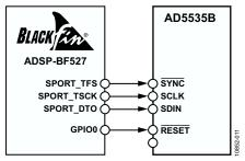
Figure 16. AD5535B-to-ADSP-BF527 Interface
