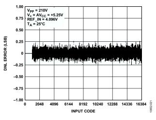
Figure 7. DNL with Full-Scale Range = 200 V
