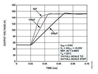
Figure 14. Settling Time vs. Capacitive Load
