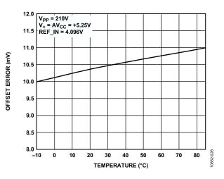
Figure 11. Offset Error vs. Temperature
