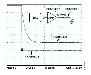
Figure 8. Short-Circuit Current Limit Timing
